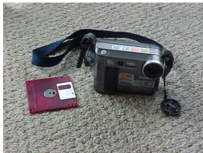
A digital camera developed by Sony Corp. in the 1990's called the Mavica records pictures in megapixels and stores them on a floppy disc for viewing on a monitor or printing photographs in gray scale, color, or sepia tone.
