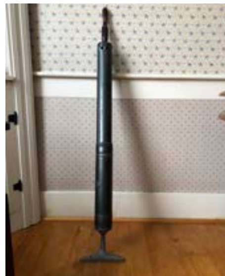
The Reeves Suction Sweeper, described as a “must for modern household sanitation,” required the operator to pump the wooden handle up and down to create a vacuum.
